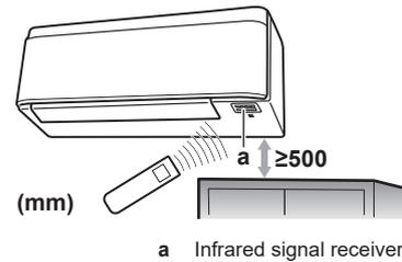
**Note:** Make sure that there are no obstacles within 500 mm under the infrared signal receiver. They may influence reception performance of the wireless remote control.
