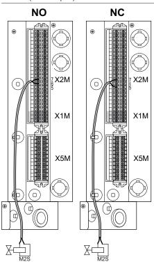
2 Fix the cable with cable ties to the cable tie mountings.
