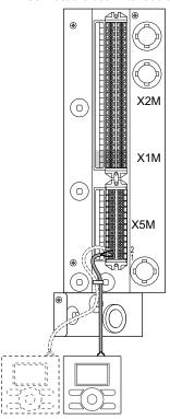
2 Fix the cable with cable ties to the cable tie mountings.
