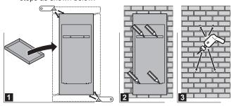
2 Fix the wall bracket to the wall with 2 M8 bolts.
