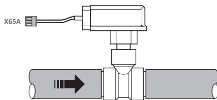
A terminal (X65A) is provided in the switch box for the electrical connection of the flowswitch (S10L).
